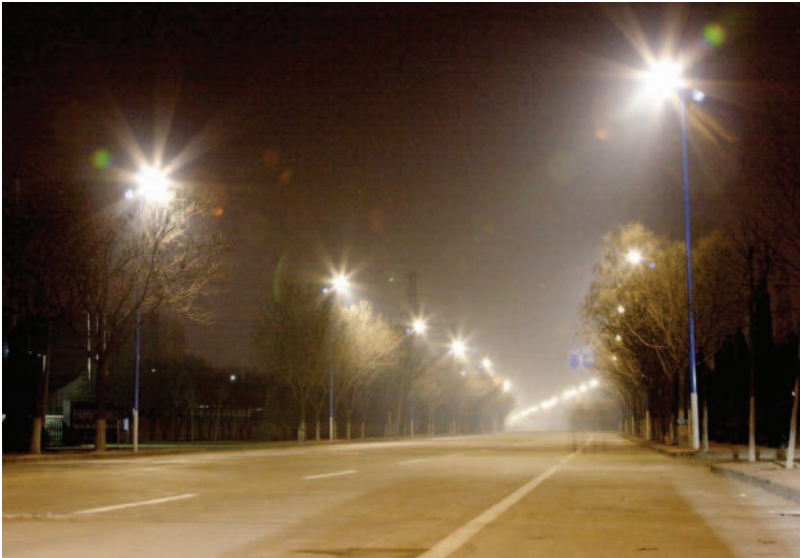
STREETLIGHTS PRODUCE A LOT OF GLARE AND UNWANTED UPWARD LIGHTING
